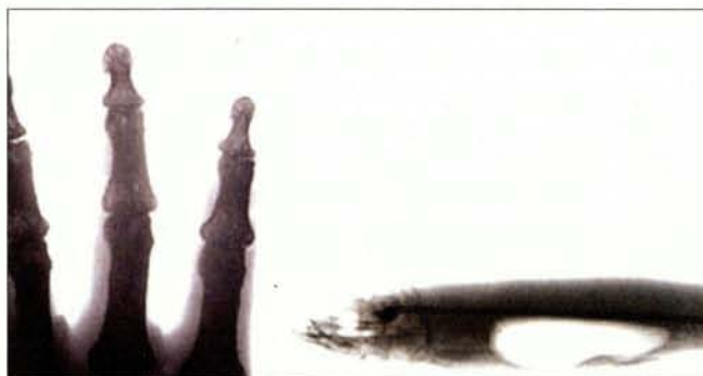
These pictures of a hand and a fish were taken with a carbon-nanotube X-ray source.
