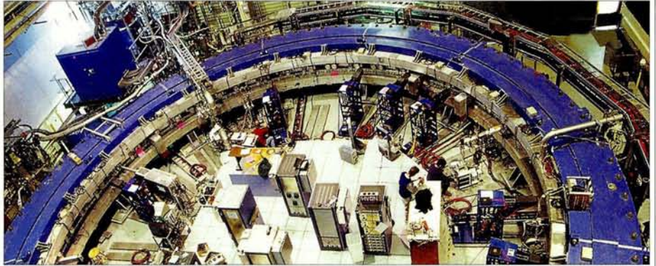
The muon storage ring used for Brookhaven's dedicated muon g-2 experiment. (BNL.)
